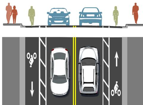
Bikes ride in buffered lane traveling in same direction as motor vehicle traffic
