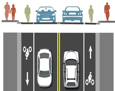
Bikes ride in separate lane traveling in same direction as motor vehicle traffic
