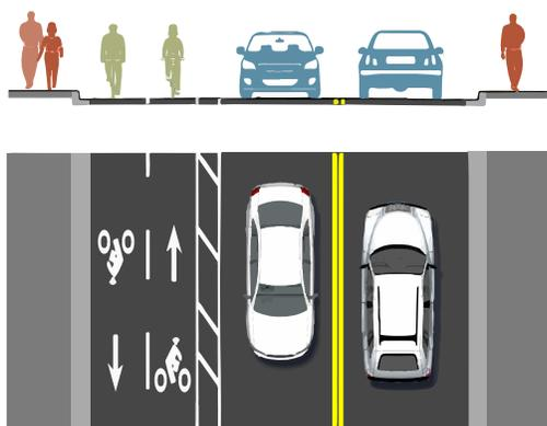
Bikes ride in both directions in separate facility adjacent to motor vehicle traffic
