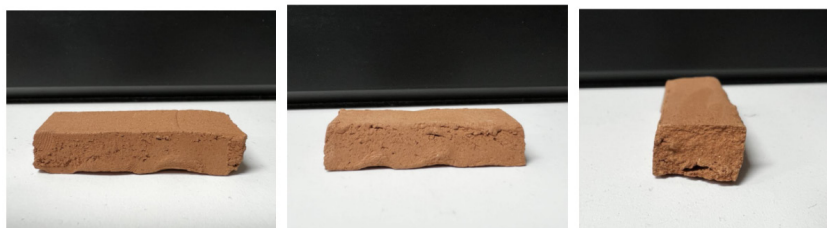
Figure 1. Imperfections in briquette morphology: A) Untempered briquette 1 with slightly warped edges on the bottom side; B) Quartz Sand-tempered briquette 1 with slightly warped edges on the bottom side; C) Untempered briquette 10 with a cavity within the body.
